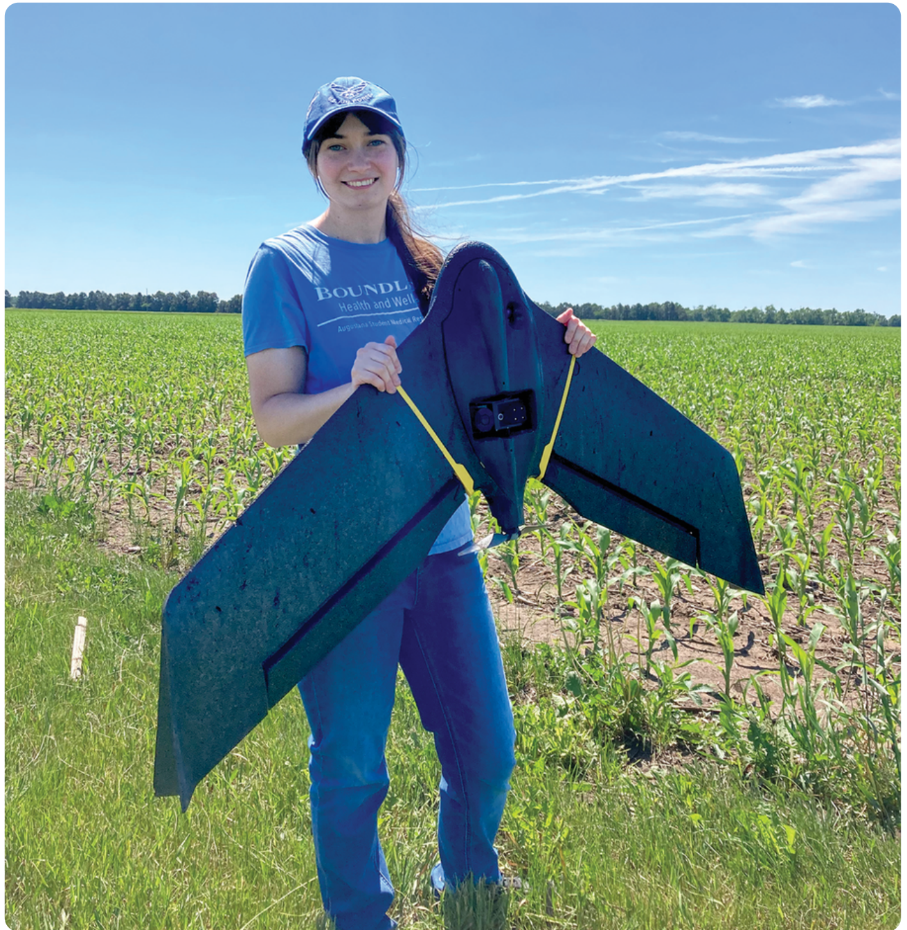
South Dakota State University graduate student Skye Brugler poses with a multispectral drone, which can be used in precision agriculture to capture imaging data and monitor plant health, productivity, stress, growth, disease, and other qualities. Photo by Deepak Joshi.
