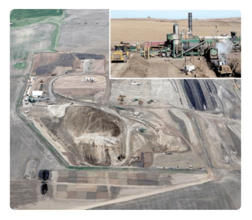
Aerial view of the oil spill remediation site and research plots with inset showing the thermal desorption unit used to treat soils during this project. Photos by Vern Whitten and Peter O'Brien.
