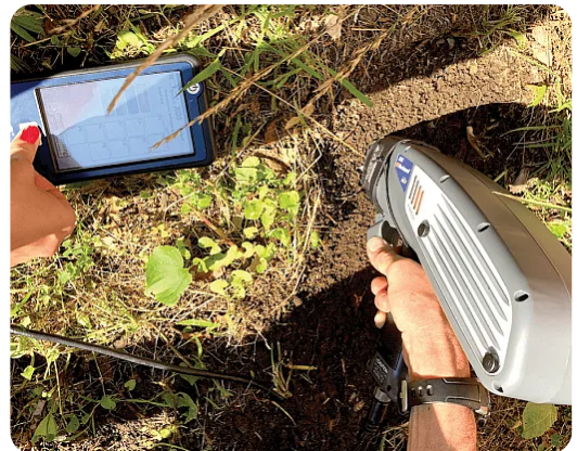
Using a handheld X-ray fluorescence (XRF) analyzer for in-field soil lead testing. Photo courtesy of Anna Paltseva.
