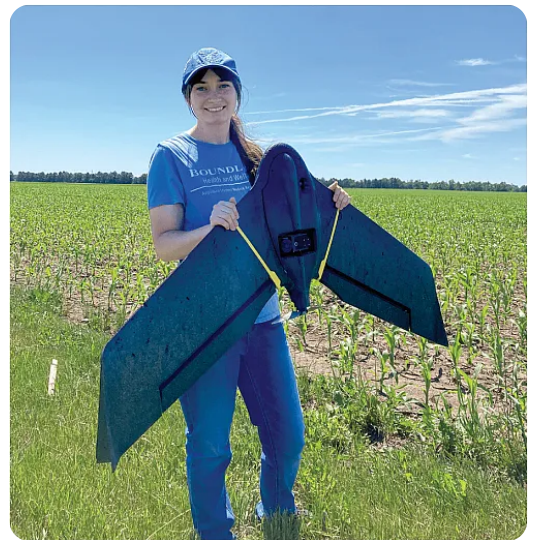
South Dakota State University graduate student Skye Brugler poses with a multispectral drone, which can be used in precision agriculture to capture imaging data and monitor plant health,
