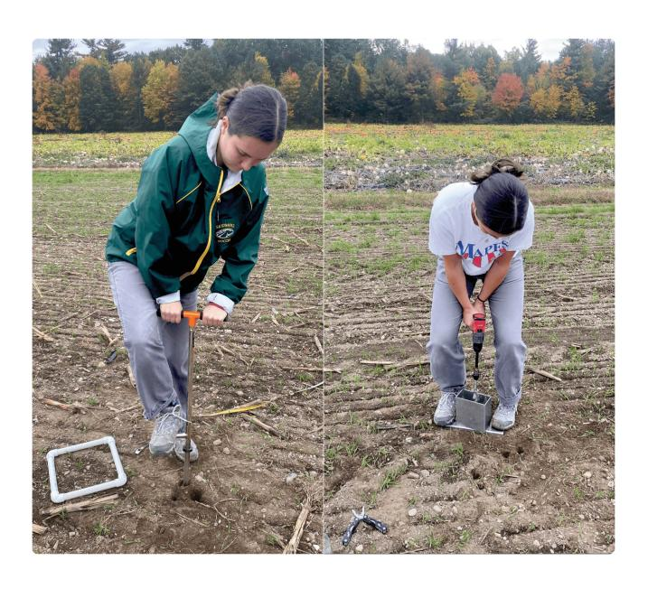
Skidmore College student Claire Wolgast collects soil samples with a traditional 1-inch push probe (left) and a novel drill-mounted auger system (right) to be analyzed for soil carbon concentration. Photos by Kelsey Jensen.
