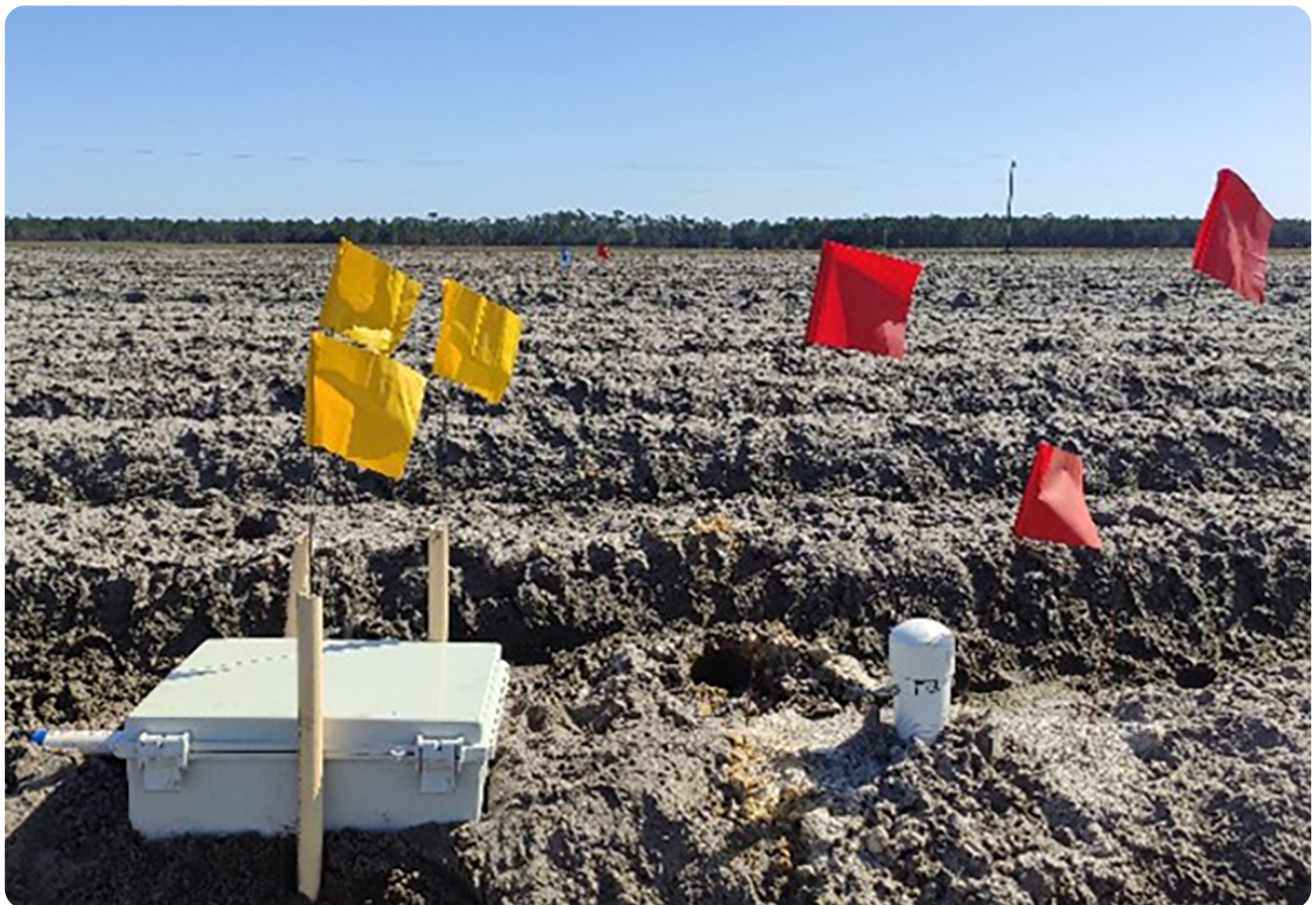
Figure 2. Soil moisture sensor in a potato field, reporting moisture at different depths at 15-minute intervals. Photo by Judyson de Matos Oliveira.
